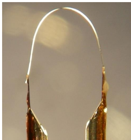
Fig. Elastically bent organic crystal.
